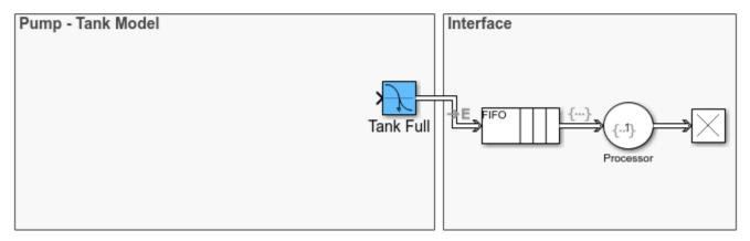
The Pump -Tank model is the Simulink component that represents the time-driven tank filling process. When a tank is full, it generates a SimEvents message through the Hit Crossing block and the message follows a similar flow of generation, queuing, service, and termination. The badge denotes the transition between time-based and event-based behavior.
