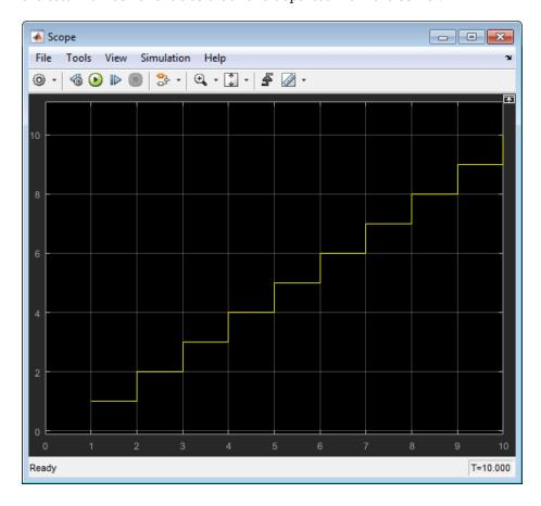
After an entity departs from the Entity Server block, the block updates its output signal at the d port.
