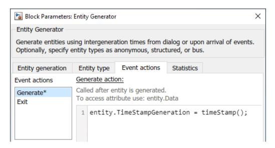
To call the function, in the Entity Generator block, in the **Event actions** tab, in the **Generate** field, use this code:
